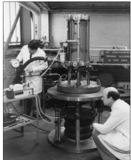
Pneumatic actuator functional test simulating increasing load over the full load.
