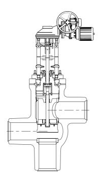
These valves can also be supplied with a direct mounted electric actuator.
