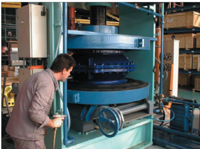
Example of a test on DN 700 (NPS 28) carried out on every single valve of our production
